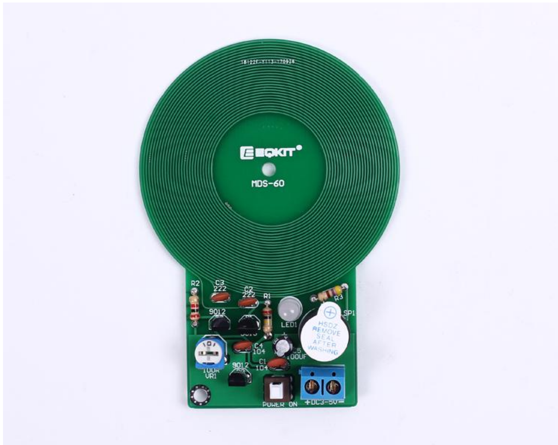
Step 5: Install Buzzer and Power socket.
