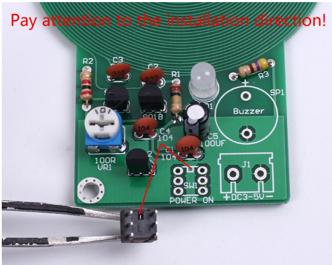
Step 4: Install power self-locking switch. Pay attention to the installation direction!!
