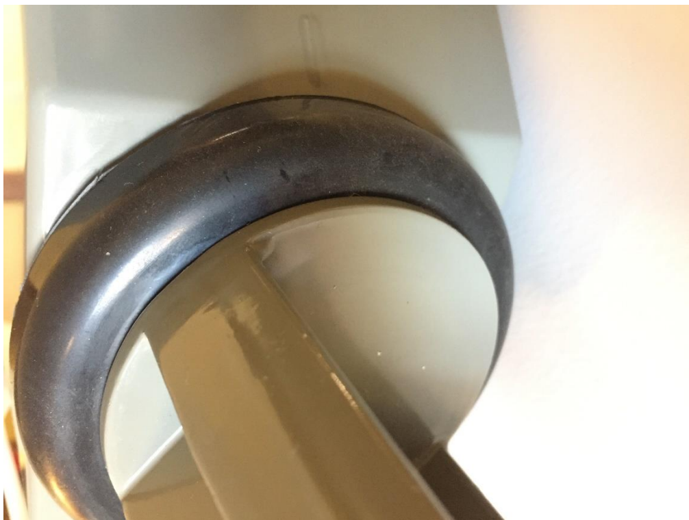
Step 1 - Remove the black, neoprene boot on the rotator shaft
