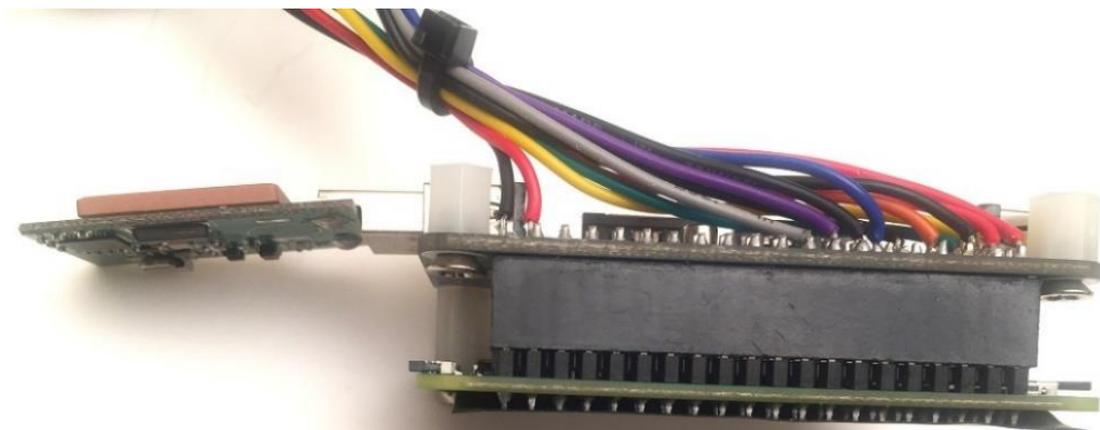
Figure 16 – RPi0 Assembly showing two 6mm spacers
