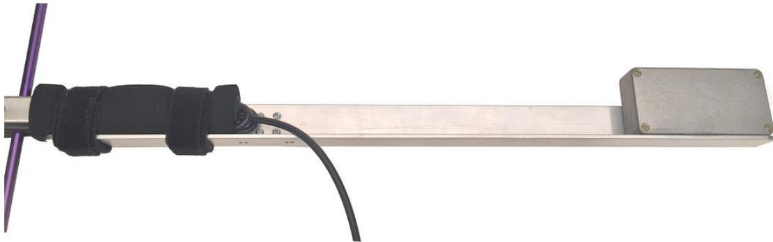
*Figure 31 – Counterbalanced Lift-arm*
