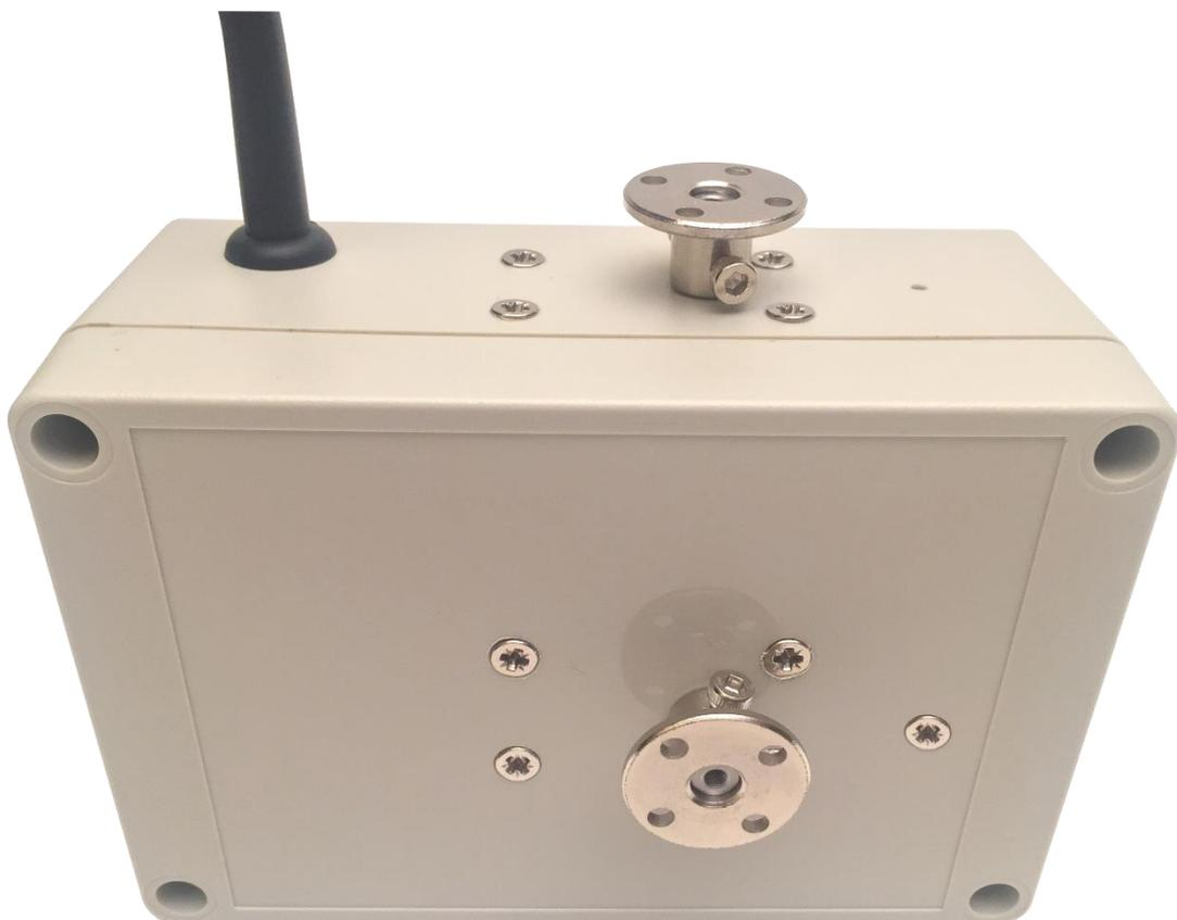
*Figure 27 – Finished unit. AZ Motor at top. EL Motor at front.*
