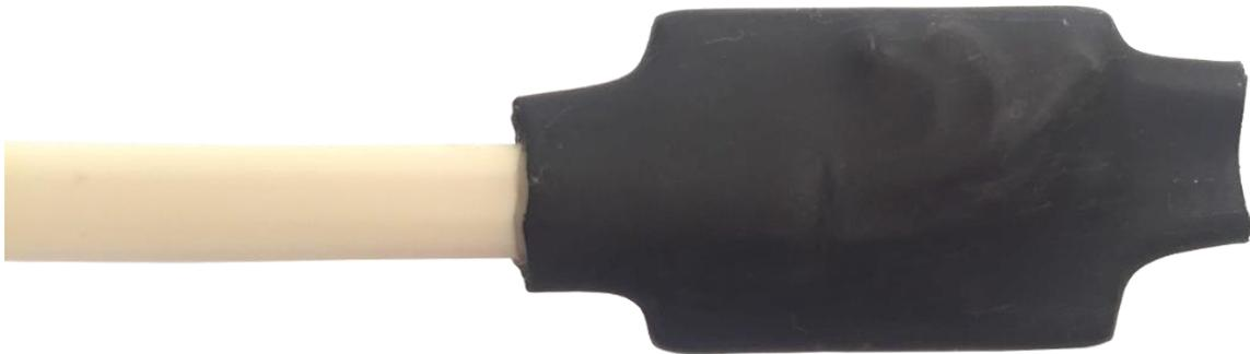
*Figure 24 – 3D Sensor with Heat-Shrink*
